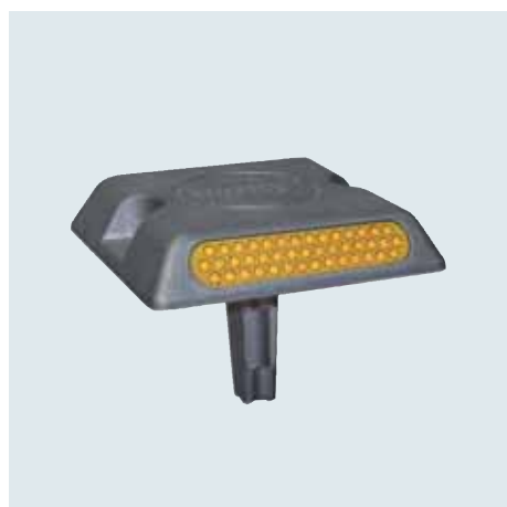
Art. 5209 one-way reflective Art. 5210 two-way reflective New body design with finger grips Dimensions: 101 x 102 x 19.8 mm Length anchoring shank: 50 mm Aluminium body with 1 or 2 x 43 glass elements
