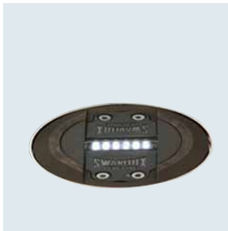
LEVELITE module 6 LEDs per side, one- or two-way Colours: white, red, yellow, green or blue Dimensions installation canister: Ø 130 mm, depth 60 mm, maximum height of LED modules above road surface: 3 mm
