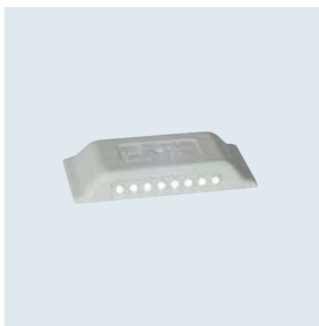
Art. 3091 one-way reflective Art. 3092 two-way reflective Dimensions: 68 x 34 x 9.8 mm Plastic body with 1 or 2 x 8 glass elements
