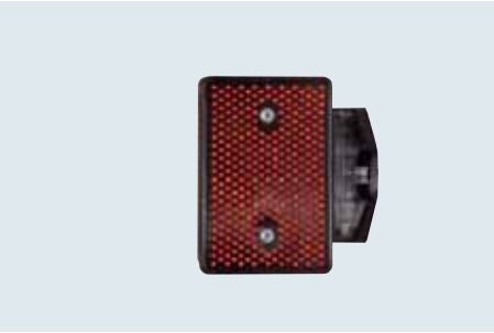
WALLFLEX SIDE Art. 5163, one-way reflective Art. 5164, two-way reflective Dimensions: 128 x 110 mm Mounting with 1 or 2 x 346 glass elements
