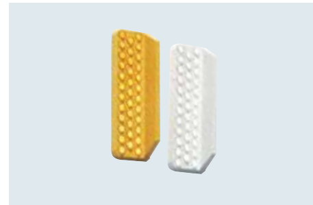
Art. 3340 Art. 3340 B (with butyl adhesive) Art. 3340 S (with two mounting holes) Dimensions: 60 x 18 x 14 mm with 35 glass elements
