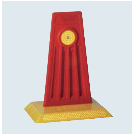
Art. 5020 two-way reflective Dimensions: 220 x 150 x 285 mm Base plate 25 mm high with 2 x 128 glass elements, rubber flag with 2 round glass reflectors
