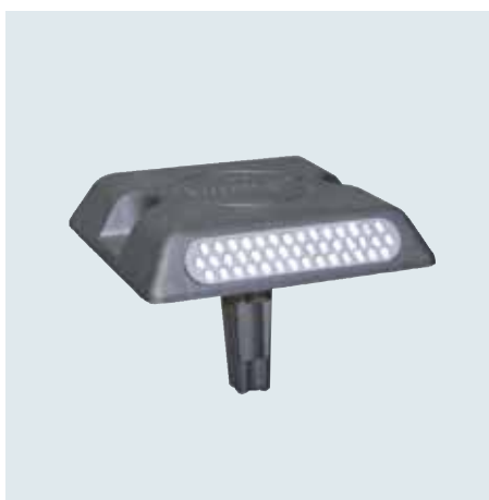
Art. 5211 one-way reflective Art. 5212 two-way reflective New body design with finger grips Dimensions: 101 x 102 x 19.8 mm Length anchoring shank: 50 mm Aluminium body with 1 or 2 x 43 glass elements, 19° tilted
