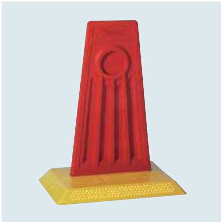
Art. 5017 one-way reflective Art. 5018 two-way reflective Dimensions: 220 x 150 x 285 mm Base plate 25 mm high with 1 or 2 x 128 glass elements, rubber flag without reflector
