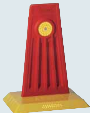
Art. 5060 two-way reflective Dimensions: 220 x 150 x 285 mm Base plate 25 mm high with 2 x 21 glass elements, rubber flag with 2 round glass reflectors
