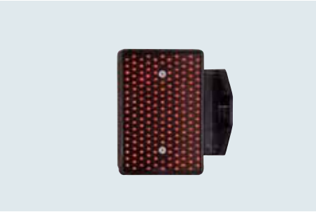
WALLFLEX SIDE Art. 5161 one-way reflective Art. 5162 two-way reflective Dimensions: 128 x 110 mm Mounting with 1 or 2 x 188 glass elements
