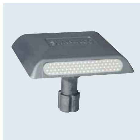
Art. 5031 one-way reflective Art. 5032 two-way reflective Dimensions: 149 x 149 x 27 mm Length anchoring shank: 80 mm Aluminium body with 1 or 2 x 76 glass elements (also available with 1 or 2 x 39 glass elements).
